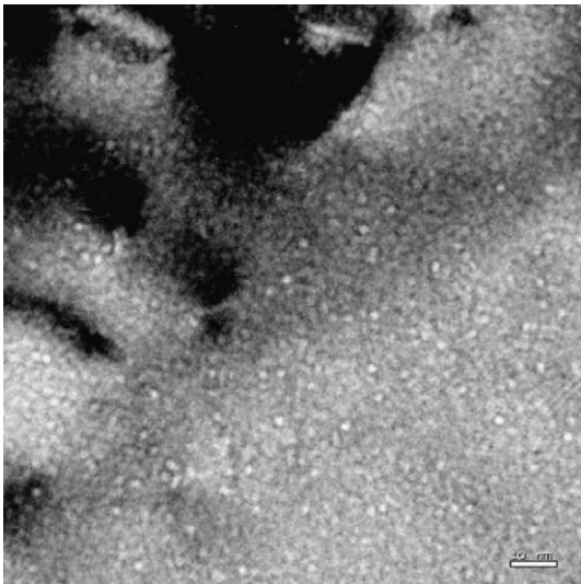
Fig. 15. TEM micrograph showing small bubbles in cold-worked EM10 irradiated at 330 °C to 10.6 dpa. Under-focus imaging conditions ( \delta f = -1000 nm). The scale bar represents 10 nm.
